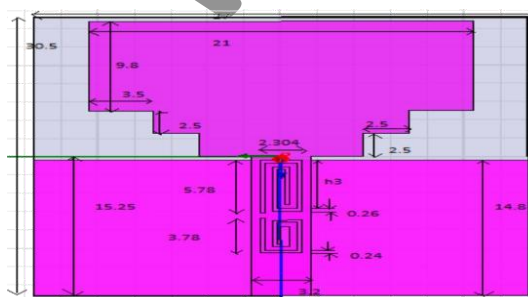
Fig. 2.1 Geometry of the Proposed Antenna
